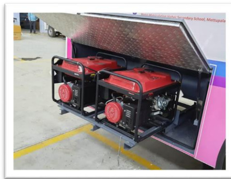
Two Generator sets, one for the mammography equipment and one for the rest of the vehicle
