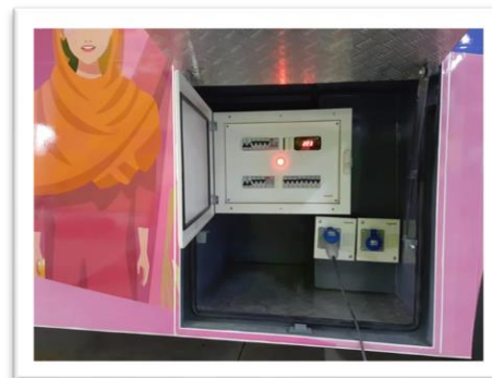
Power Distribution Box, with the option to use external single phase AC input
